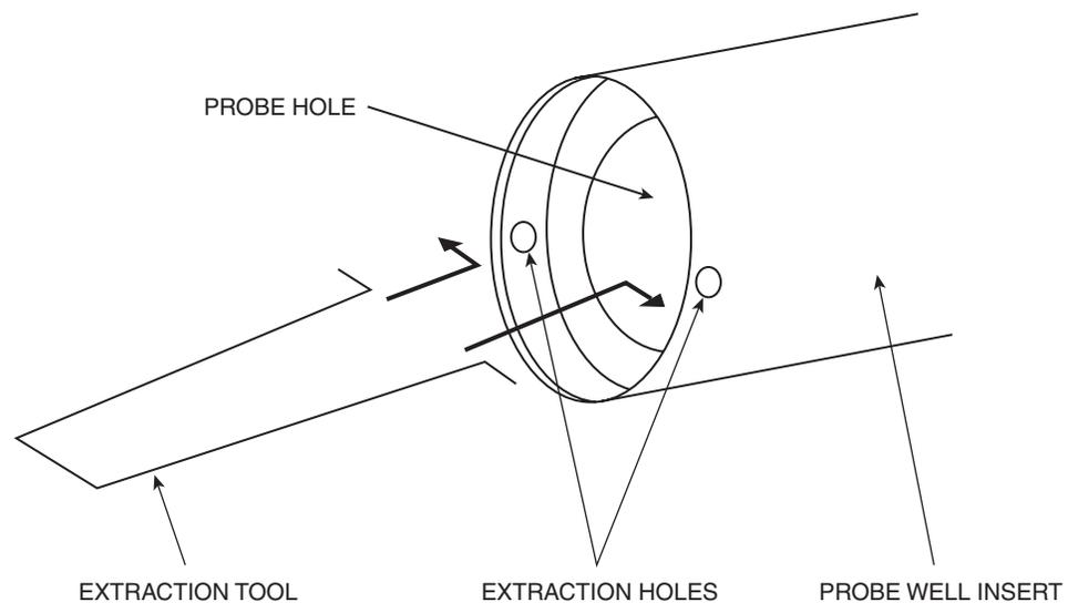
Figure 10. Removal of Probe Well Insert in CL900A
