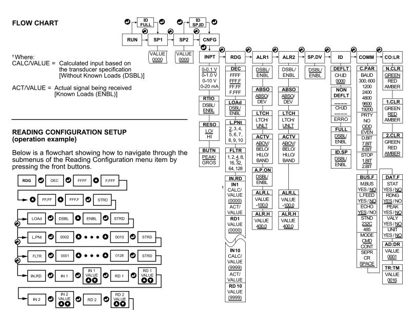
Above is a flowchart showing how to navigate through all top level menus by pressing the 2 and 5 buttons.
