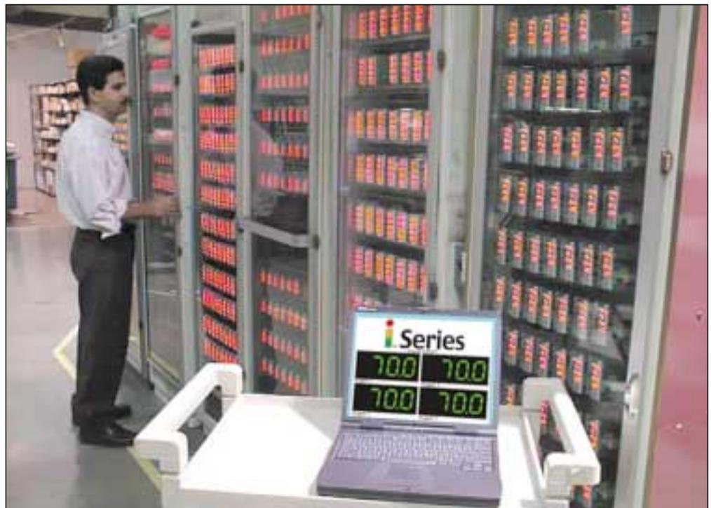
*Burn-in ovens at NEWPORT are monitored and controlled by the test engineering dept. over an Ethernet LAN. The printed circuit board assemblies for all NEWPORT products go through a 24-hour burn-in and thermal cycling prior to test and calibration.*
