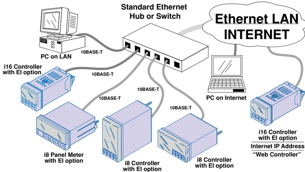
Meters and controllers connect directly to an Ethernet LAN or Internet as nodes on the network, same as a PC.
