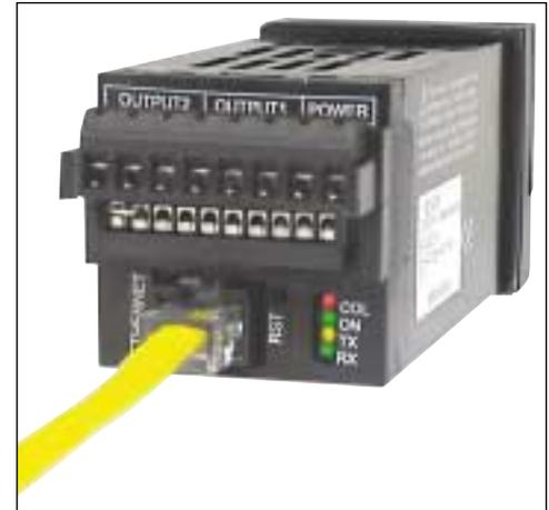
*Devices as small as 1/16 DIN temperature controllers (48mm x 48mm panel cutout) can be connected directly to an Ethernet LAN and the Internet.*
