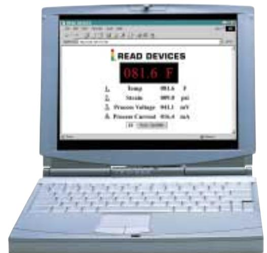
*Controllers and meters with Embedded Internet can serve Active Web pages to any computer on an Ethernet LAN or the Internet.*
