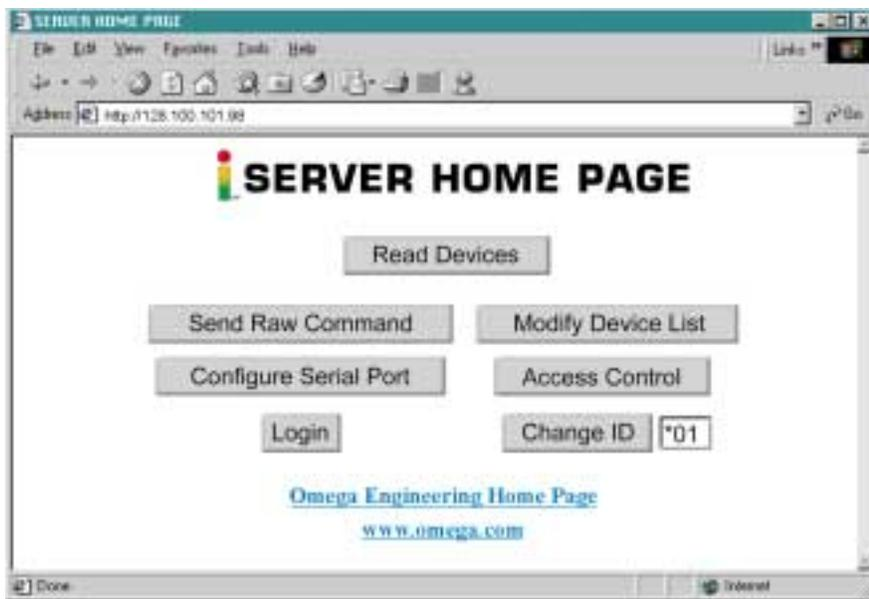
*Devices with Embedded Internet can serve Active Web pages to any computer by typing the IP address or unique name in a Web browser.*
