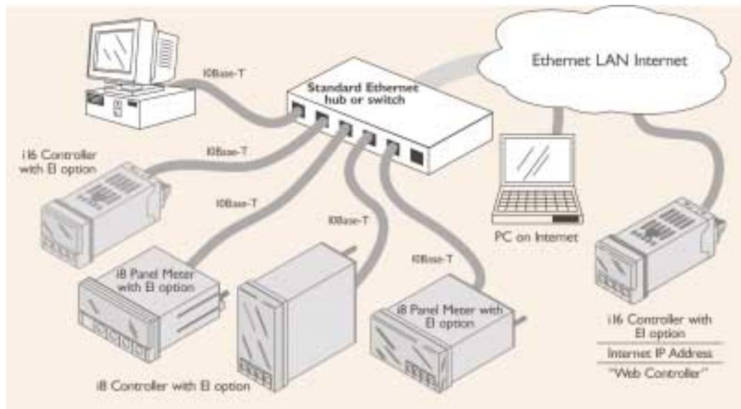
Fig 2 Direct connection to Ethernet LAN or Internet
