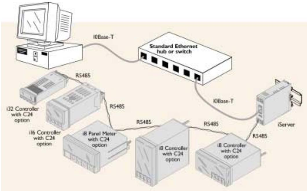
Fig 3 Integration of server controller hub for up to 32 devices
