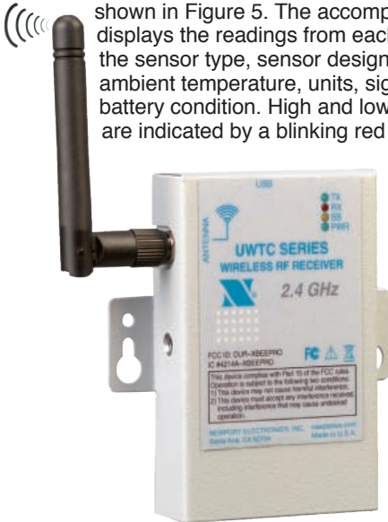
Figure 5 – UWTC REC1, wireless 12-channel USB receiver.
